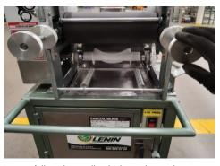
Adjust the gordita thickness by turning the adjustment knobs (clockwise to make the tortilla thinner, and counter clockwise to make it thicker) Lower the clutch lever when you obtain the desired thickness
