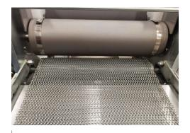
Check that the straps rotate freely
