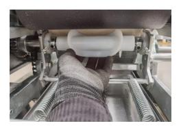
Place cutter on the base, verify that it is correctly installed and secured
